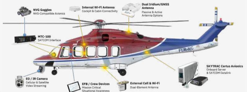
Figure 4. Critical components relying on Satcom on a modern SAR helicopter.
