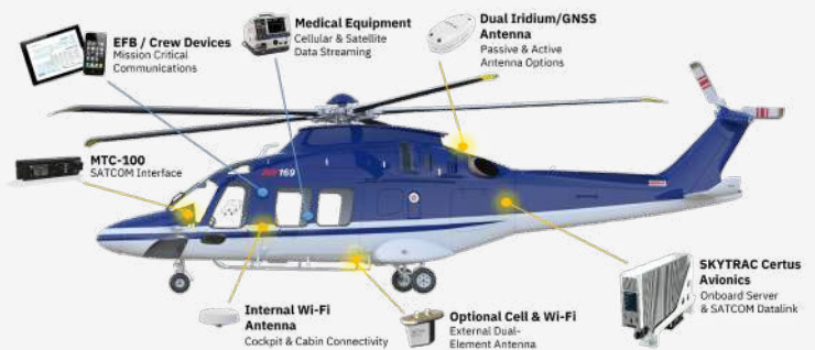
Figure 3. Critical components to enable onboard medical data transfer.
