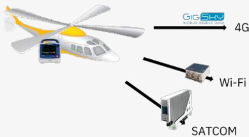
Figure 5. SKYTRAC pipelines for data offloading.
